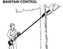
· Keep a good, firm grip on the pruner with both hands when the engine is running and don't let go. A firm grip will help you reduce kickback and maintain control. Keep the fingers of your left hand encircling and your left thumb under the assist handle. Keep your right hand completely around the throttle handle whether your are right handed or left handed.
